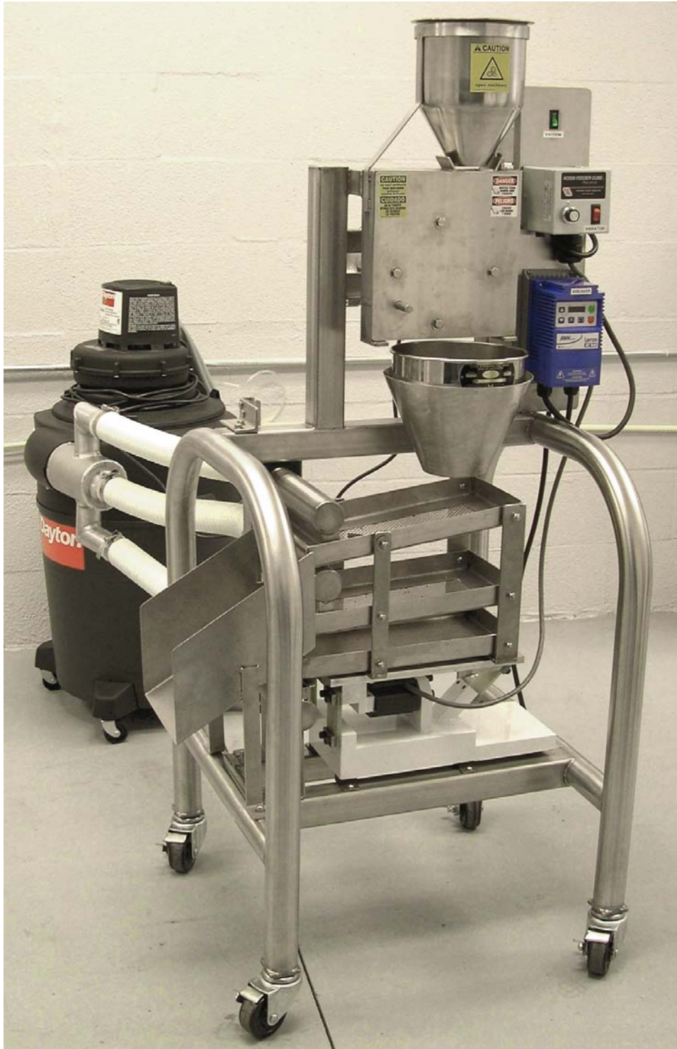
Winn-15 Mini Cocoa Bean Winnower. Shown with Optional Variable Speed Bean Breaker.
