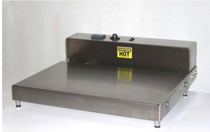
T400CC - Standard Bench Top Tempering/Mixing Table Electrically Heated and Water Cooled - Work Surface 15 in. by 22 in. Note Water Inlet/Outlet on Right Side of Work Surface
